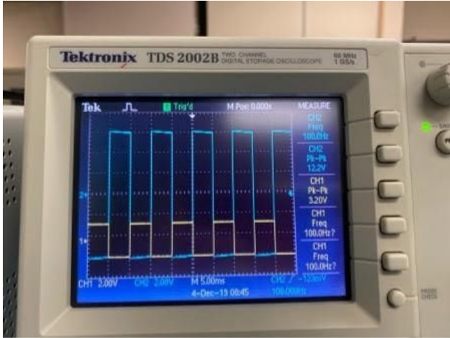
Figure 3: Level Shifter Waveform
